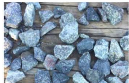
Large Cuttings Are Very Difficult To Remove.
