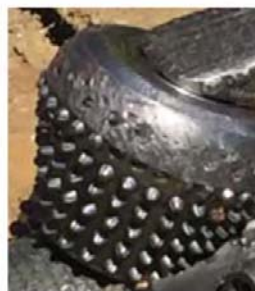
Damaged From Loose Cuttings.
